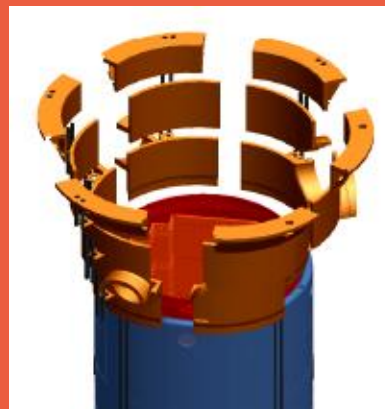
Dismantling the internal parts with band saw at Stade nuclear power station, Germany
